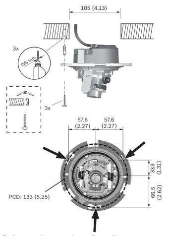
To flush mount the camera in a wall or ceiling:
